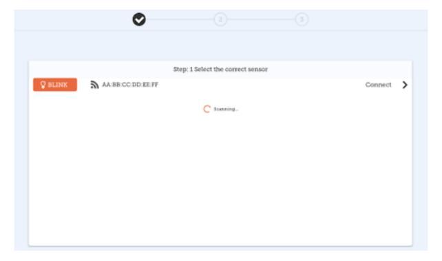
If you tap the **BLINK** button, the LED light for that sensor will flash. You can use this to make sure that you are connecting the correct sensor.
