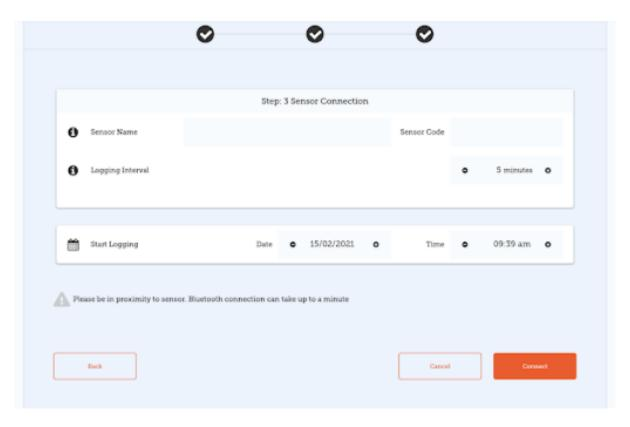
Tap **Back** if you wish to return to Step 2 and edit the sensor thresholds (temperature breach conditions). Tap **Connect** to complete sensor setup and add the sensor to mSupply mobile. This will return you to the mSupply mobile vaccine home screen and you will see the sensor has been added.
