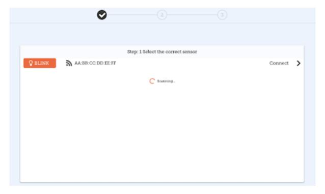
If you press the BLINK button, the LED light for that sensor will flash. You can use this to make sure that you are connecting the correct sensor.
