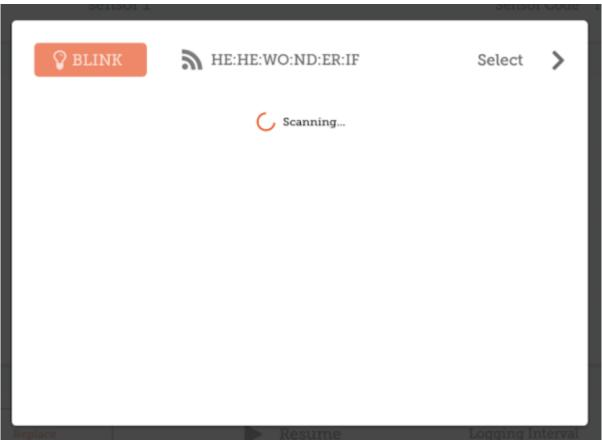
From the list, select the replacement sensor. You can press Blink to check that you have the correct sensor (the LED light will flash for this sensor).
