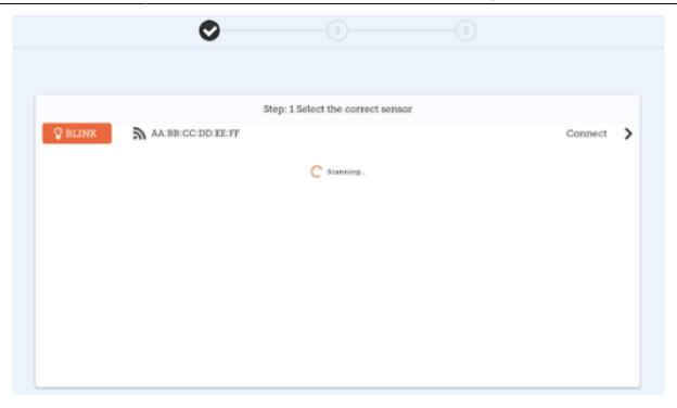
If you tap the **BLINK** button, the LED light for that sensor will flash. You can use this to make sure that you are connecting the correct sensor.
