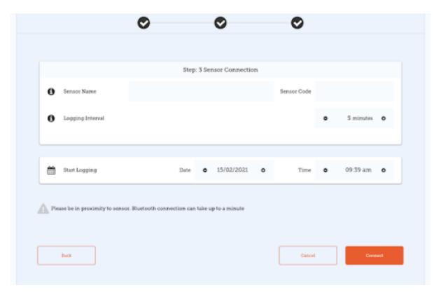
Tap **Connect** to complete sensor setup and add the sensor to mSupply mobile. This will return you to the mSupply mobile vaccine home screen and you will see the sensor has been added.
