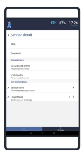
Blink: Pressing here will cause the sensor light to flash. You can use this feature to ensure that you
