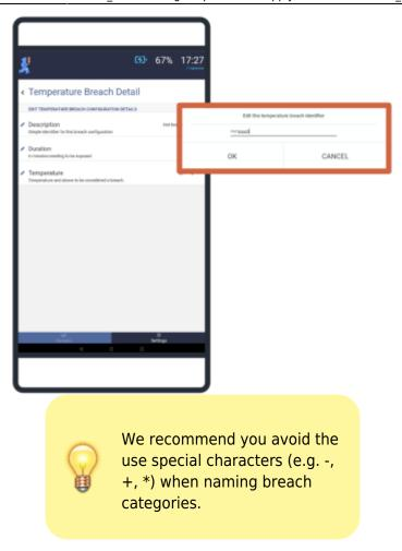
**Duration:** Using the slider, you can determine how long the temperature must continuously remain outside of the required temperature range for it to be considered a breach. You can set the duration to any length between 1 and 600 minutes.
