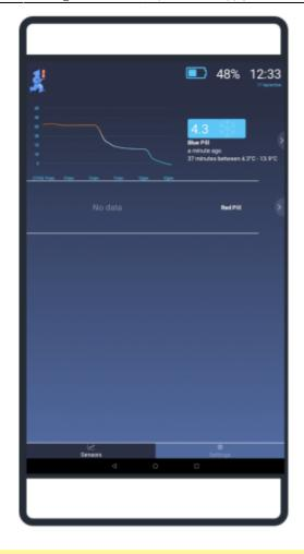
When a sensor is first linked and no temperatures have been logged, the graph will display with no data (as above for Red Pill). The graph will update when there are two temperature logs.
