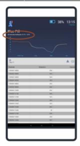
The new date range will also be used as the time period to calculate cumulative temperature breaches. If there has been a cumulative temperature breach during this period (using the temperature and duration settings in the cumulative exposure breach settings, the cumulative breach indicator/text will be displayed underneath the sensor name.
