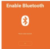
If the device is turned off, mSupply ColdChain is closed, or Bluetooth is disabled, the sensor will store up to 20,000 temperature logs as per the sensor settings. After 20,000 logs, the sensor will overwrite the oldest logs. When the device, mSupply ColdChain application or Bluetooth is enabled again, please allow a few log intervals for transfer of all saved logs.
