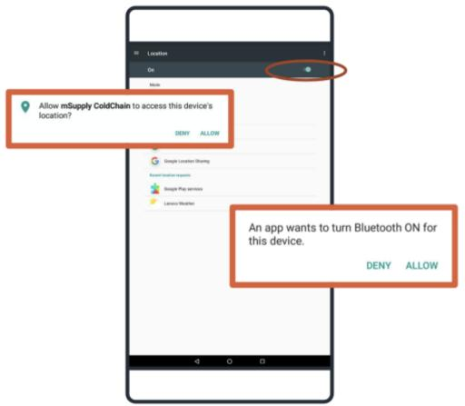
Once a sensor is linked to mSupply ColdChain, it will be automatically synchronised via Bluetooth according to the user-programmable schedule. mSupply ColdChain requires Bluetooth to be enabled in order to receive temperature logs. If Bluetooth is disabled when the application is operating, the user will be prompted to reconnect.
