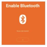
If the device is turned off, mSupply ColdChain is closed, or Bluetooth is disabled, the sensor will store up to 20,000 temperature logs as per the sensor settings. After 20,000 logs, the sensor will overwrite the oldest logs. When the device, mSupply ColdChain application or Bluetooth is enabled again, please allow a few log intervals for transfer of all saved logs.
