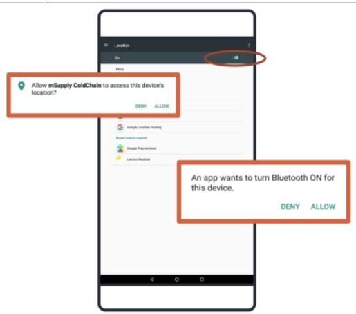
Once a sensor is linked to mSupply ColdChain, it will be automatically synchronised via Bluetooth according to the user-programmable schedule. mSupply ColdChain requires Bluetooth to be enabled in order to receive temperature logs. If Bluetooth is disabled when the application is operating, the user will be prompted to reconnect.
