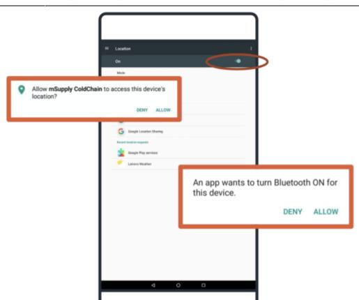
Once a sensor is linked to mSupply ColdChain, it will be automatically synchronised via Bluetooth according to the user-programmable schedule. mSupply ColdChain requires Bluetooth to be enabled in order to receive temperature logs. If Bluetooth is disabled when the application is operating, the user will be prompted to reconnect.
